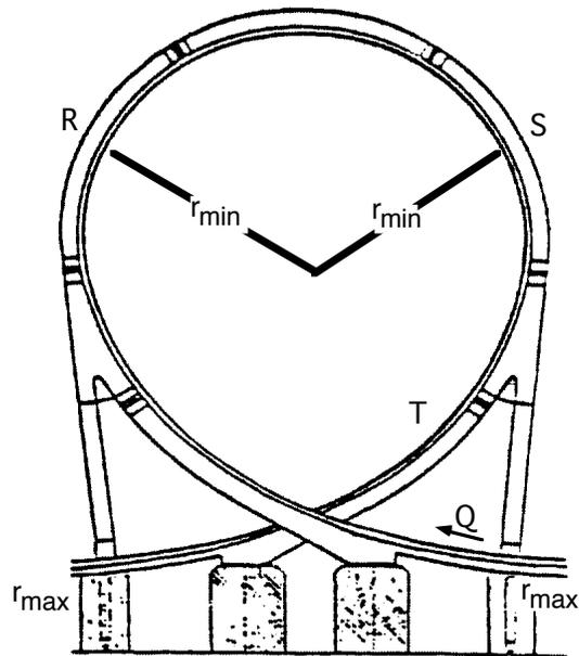
14. Accelerometers mounted in the front and rear cars to a coaster can be used to measure the force component perpendicular to the rider's seat as the coaster travels through a clothoid loop. The table below gives those data recorded for this situation. Use these data to answer the questions that follow.
